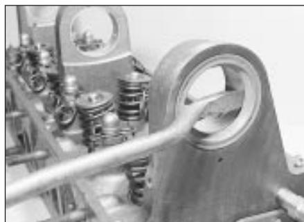
24.9 Prising out the camshaft oil seal
