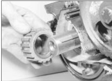
19.11 Removing the crankshaft sprocket
