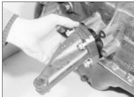
18.10a Removing the right-hand engine mounting bracket
