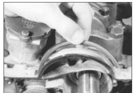
29.15b . . . then fit the rubber sealing strips
