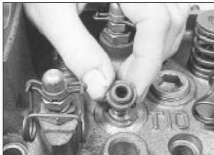
22.4 Removing a valve stem oil seal
