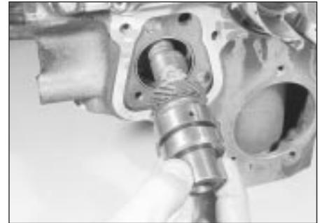
25.5b Withdraw the auxiliary shaft
