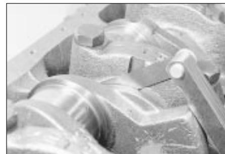
34.6 Checking crankshaft endfloat
