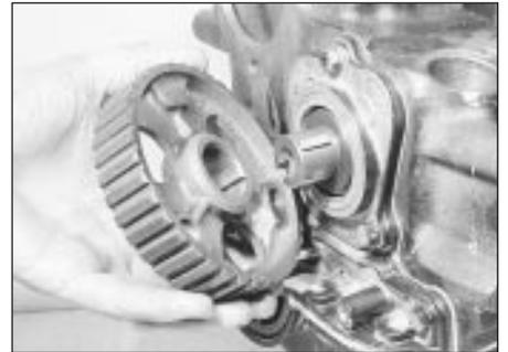
19.13 Removing the auxiliary shaft sprocket
