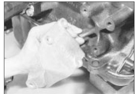
18.10b Removing the alternator mounting bracket
