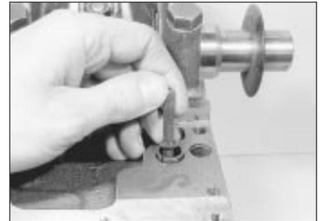
30.4 Withdrawing the oil pump driveshaft
