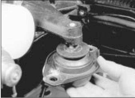
17.4 Withdrawing an engine mounting
