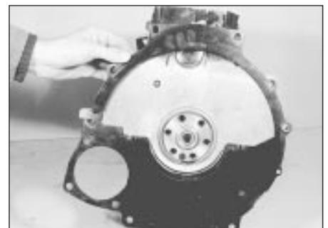
26.5 Withdrawing the engine adaptor plate
