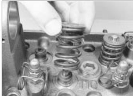
22.2b Removing a valve spring and cap
