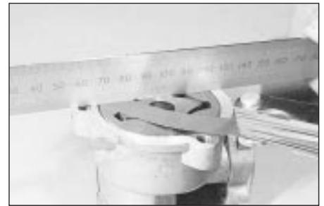
31.11 Checking the oil pump rotor endfloat
