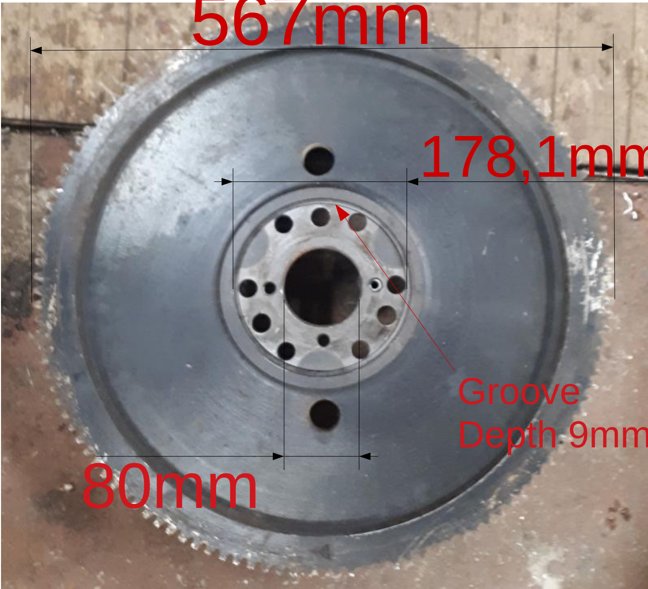
Back side of the flywheel
